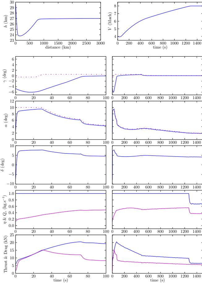
Fig. 4. Stabilisation of a representative nonlinear vehicle using the control law  $\phi_q(V, \gamma, l, q)$ .
