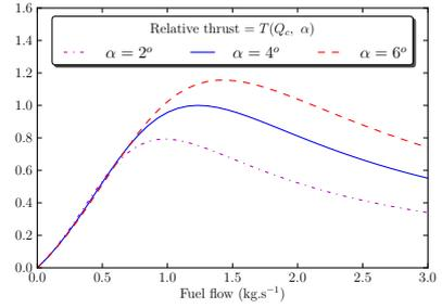
Fig. 3. Thrust force variation with respect to angle of attack and fuel flow rate.
