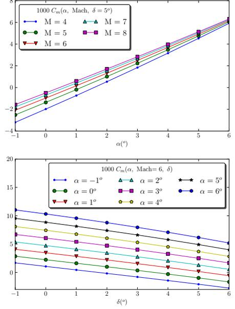
Fig. 2. Aerodynamic moment coefficient with respect to angle of attack, angle of elevators, and Mach number.
