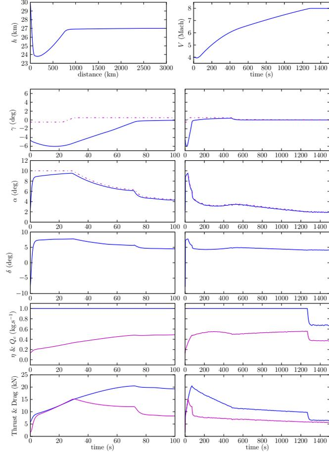
Fig. 5. Stabilisation of a representative nonlinear vehicle using the control law (49).
