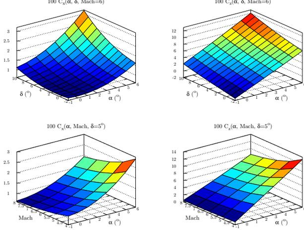
Fig. 1. Aerodynamic forces coefficients with respect to angle of attack, angle of elevators, and Mach number.
