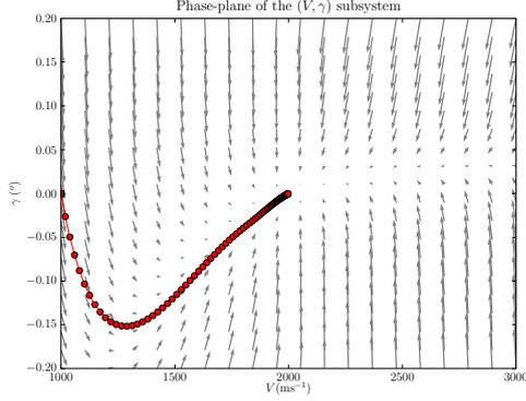
Fig. 4. Phase plane of the controlled  $(V, \gamma)$  subsystem, with reference  $(V_c, \gamma_c) = (2000, 0)$ , saturations  $(\bar{l}, \bar{l}) = (-\frac{1}{2}l_c, 2l_c)$  and  $(\bar{t}, \bar{t}) = (0, 2t_c)$ , and gains  $(k_l, k_t) = (10^{-8}, 4 \cdot 10^{-3})$ .
