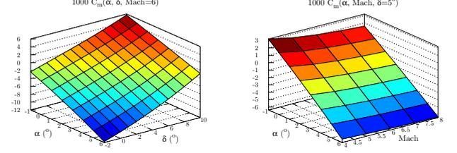
Fig. 2. Aerodynamic moment coefficient with respect to angle of attack, angle of elevators, and Mach number.
